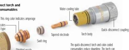
consumables reduce downtime. The torch can be installed or changed in seconds. Color-coding on consumables matches screen options to quide operators quickly through the change-over.
