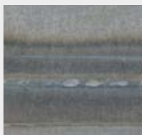
/ Dip-transfer arc I: 97 A, U: 18.1 V
