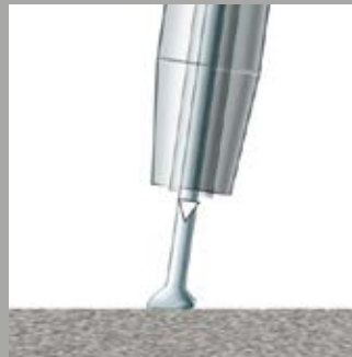
/ When the filler metal dips into the weld-pool, the arc is extinguished. The welding current is lowered.
