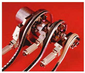
GTAW (TIG) weldable materials. Root passes may be done fusion-only, with filler wire, or with the use of insert rings. Autogenous welds (without filler metal) with 100% penetration may be done on wall thicknesses up to 0.154" (3,9 mm) depending on the alloy.
