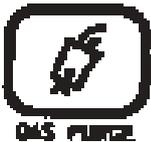
Gas purge key energizes the solenoid valve but not the wire feeder or power source
