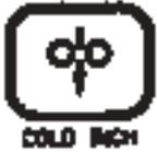
Cold Inch key energizes the wire feeder but not the power source or solenoid valve. Wire feeds at Inch speed setting. (See operating instructions, Section entitled “Display Control Keys”).
