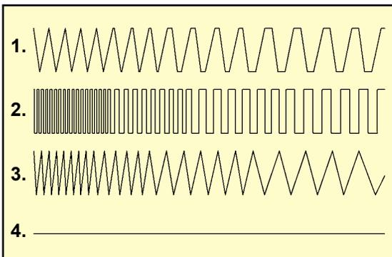
1. **RUN:** In this mode, power to the drive unit is always on and the machine travels continuously both during weave and dwell. Weave speed and dwell time both affect the weld pattern.
