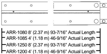
**SEMI-FLEX RAIL AFR-3000** can be flexed inside or outside to a minimum radius of 15' (5.0 m) or 30' (10.0 m) diameter without permanent deformation.
