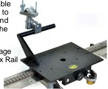
**Hi-Flex Rail (FMD)** can flex from a straight to a 30" (760 mm) radius inside or outside. The rail is made from a tempered, wear resistant, stainless steel with a steel rack. It is designed for use with the FMD Hi-Flex Carriage. The rail comes in 57.7" (1.47 m) lengths and can be held in place with magnets or vacuum cups. An optional stiffener can be installed behind the rail for heavy duty, straight line applications.
