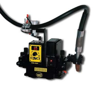
The Bug-O Systems Mini-Vert III is held on the workpiece with strong permanent magnets. It will travel and carry a welding gun in flat or vertical positions producing continuous uniform fillet welds. The Mini-Vert III features a quick torch mount which allows the welding gun to be rapidly moved from one side of the machine to the other, enabling the operator to weld the entire work piece from end to end. The Mini-Vert III is shipped with one (1) battery and one (1) battery charger.
