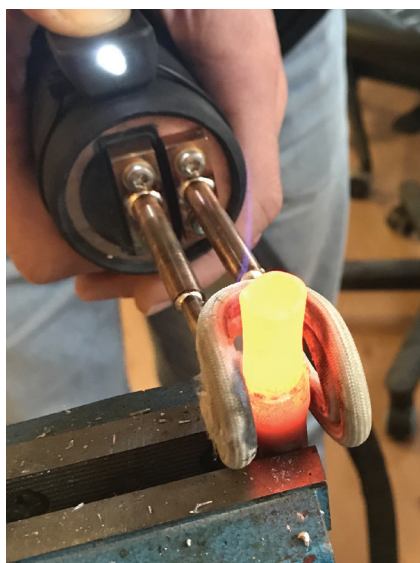
Induction soldering of copper tubes with silver solder.
