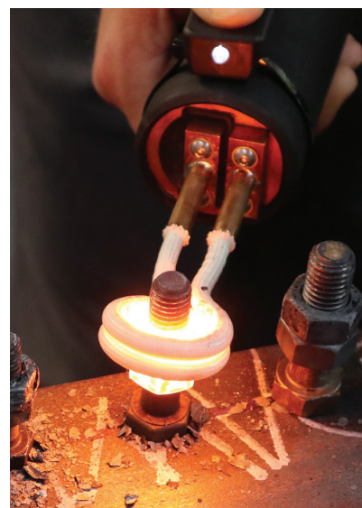
Induction heating of metal parts with round coil.
