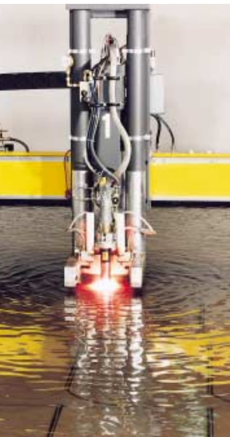
Water-injection plasma cutting
