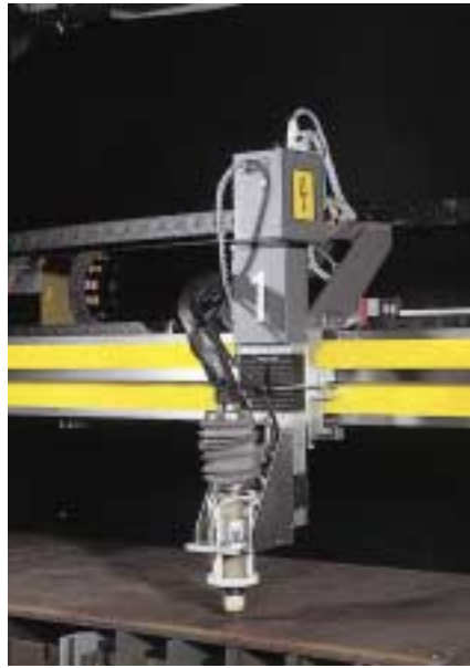
Carriage for plasma cutting
