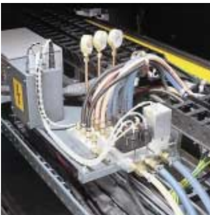
Gas supply is controlled by proportional valves
