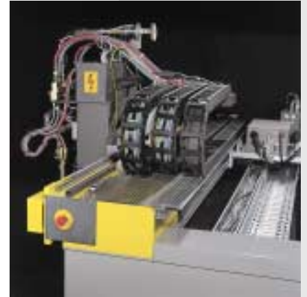
Cable chains ensure precise movement of all cutting tools
