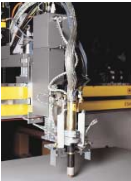
Carriage fitted with plasma cutting torch
