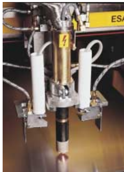
Plasma cutting with inductive initial height setting
