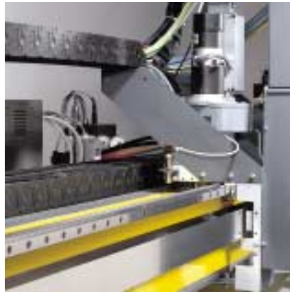
Precise linear guidance of cutting tools (option)
