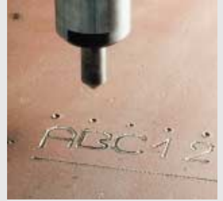
Pneumatic marking Compressed air punching
