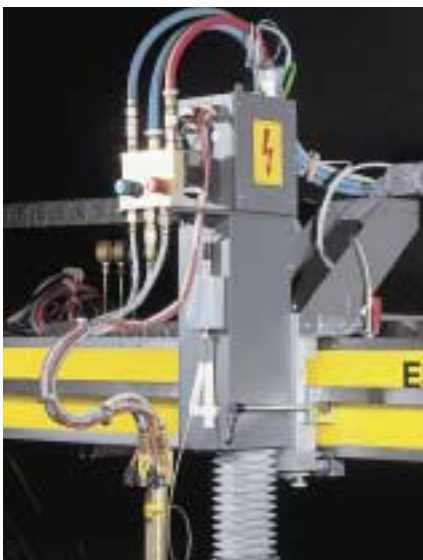
Multijet torch with automatic internal ignition
