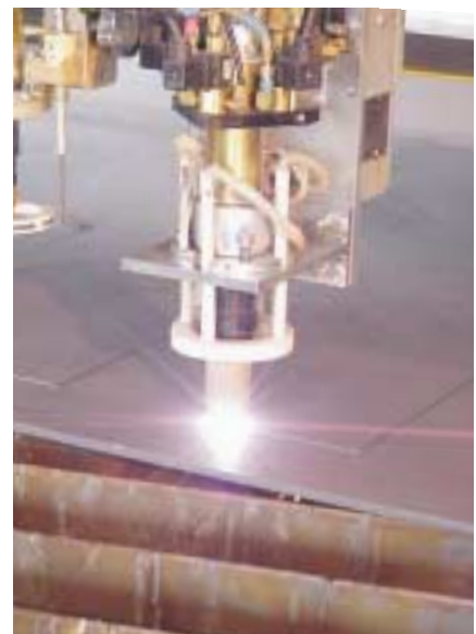
Plasma cutting with capacitive initial height setting
