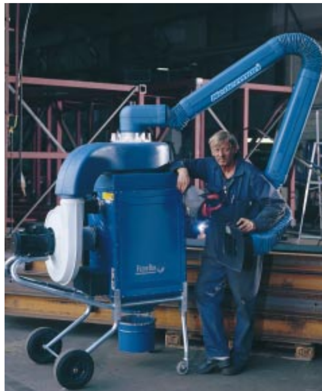
For users working with fume and dust particles that are difficult to remove, i.e. from production welding, the Filterbox with a compressed air unit is used.
