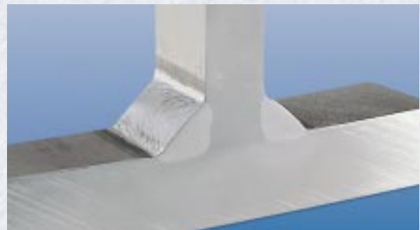
Base metal: AlMg 3 Sheet thickness: 25 mm Filler metal: AlSi 5, Ø 1.2 mm Shielding gas: Argon
