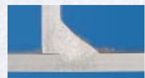
With start-up program – no fusion defects
