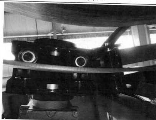
Adjustable drive wheels for inside/ outside welding
