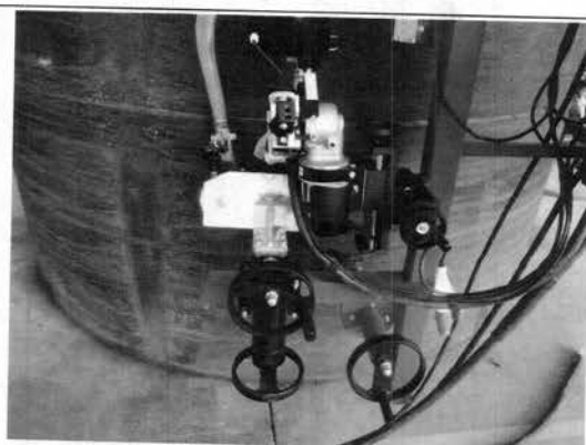
Torch, manual slide & head assembly/Lincoln NA3 head
