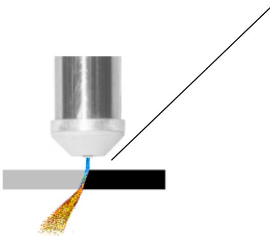
Under normal cutting conditions the torch is designed to operate with a STAND OFF of about 6 mm (except P50 8 mm). This is the distance between the end of the nozzle and the work piece.
