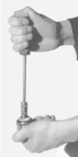
3. Unscrew the Nozzle with the special tool supplied. (See illustration left).
