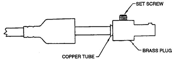
5. Tighten set screw to collapse copper tube. Screw must apply pressure against welding cable. The top of the set screw will be well below the surface of the brass plug after tightening.
