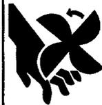
7.d. Keep all equipment safety guards, covers and devices in position and in good repair. Keep hands, hair, clothing and tools away from V-belts, gears, fans and all other moving parts when starting, operating or repairing equipment.
