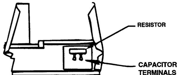
3. Use a DC voltmeter to check that voltage is not present across either capacitor.
