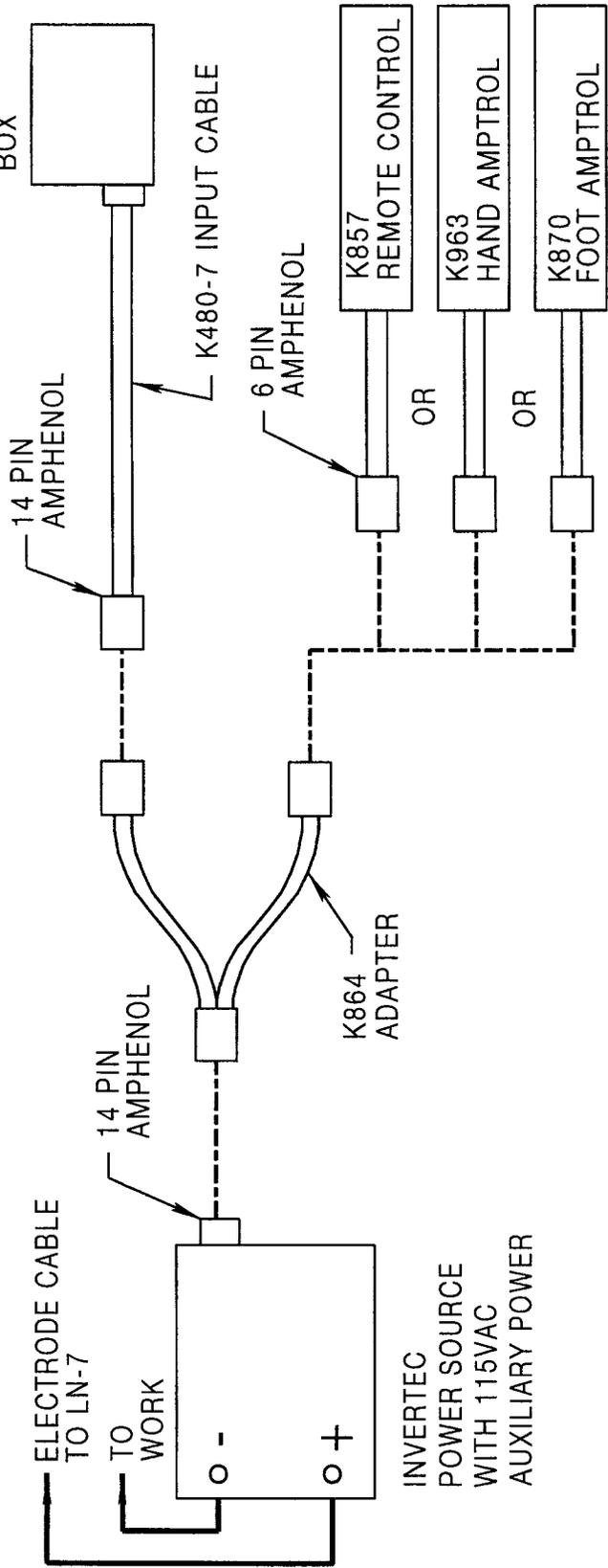
N.A. WELDING CABLE MUST BE SIZED FOR CURRENT AND DUTY CYCLE OF APPLICATION.
