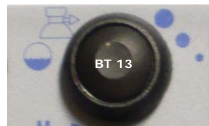
Fig. 5.4 - Push button for gas flow test - cooling system test - and manual start of the coolant pump
