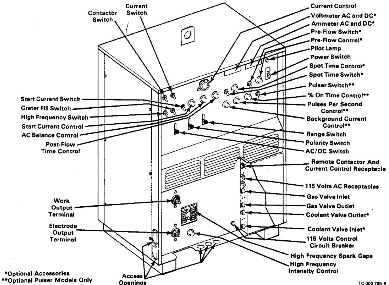
Figure 4-1. Front Panel View (300 Ampere Model Illustrated)
