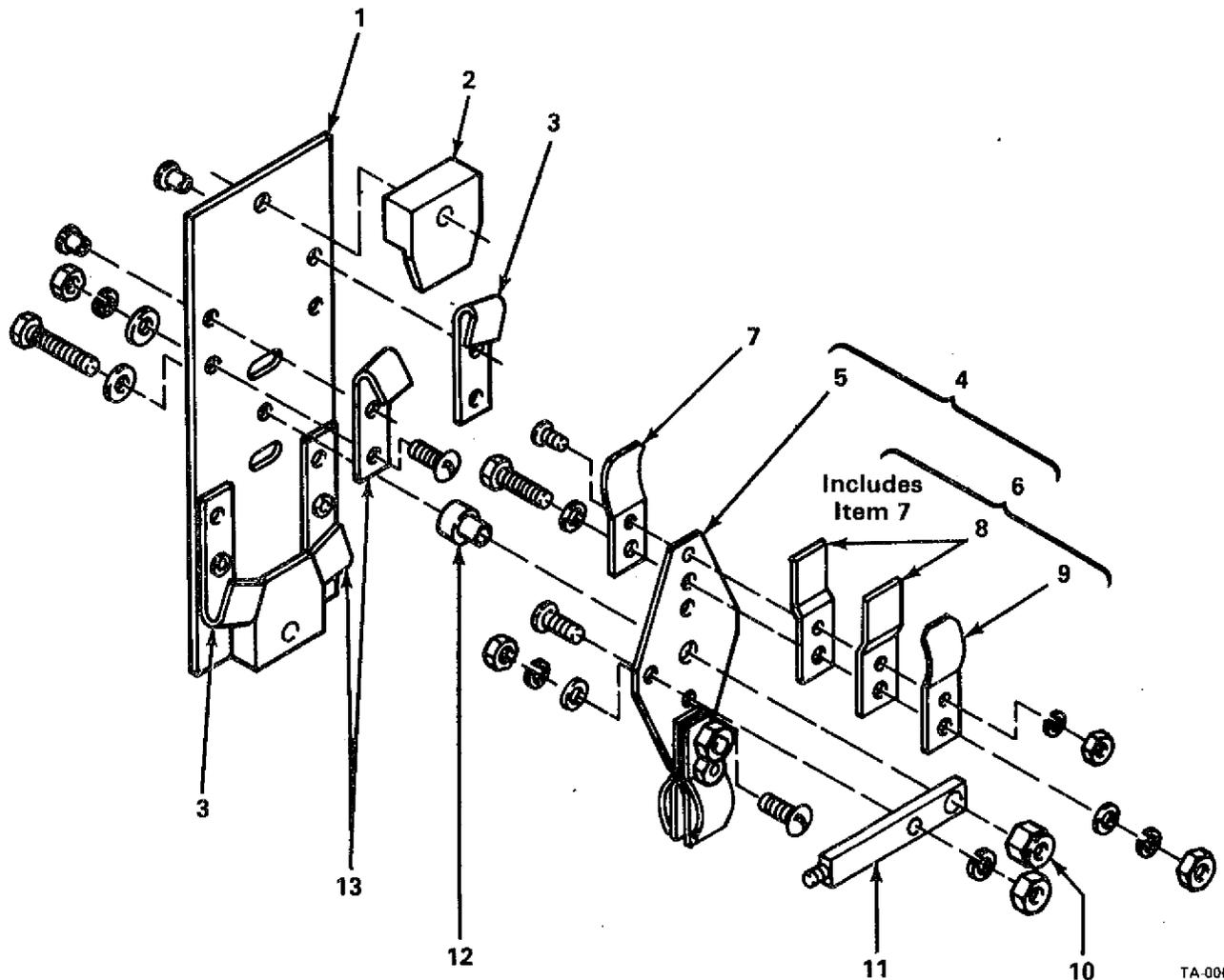
Figure G1D - Contact Board, Switch-Range
