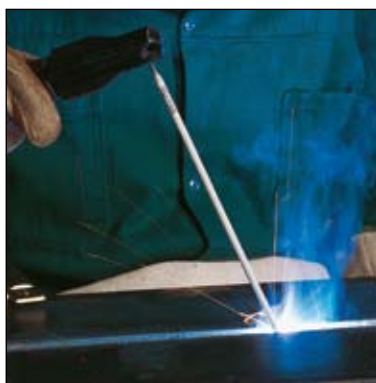
MMA in a V-joint.
