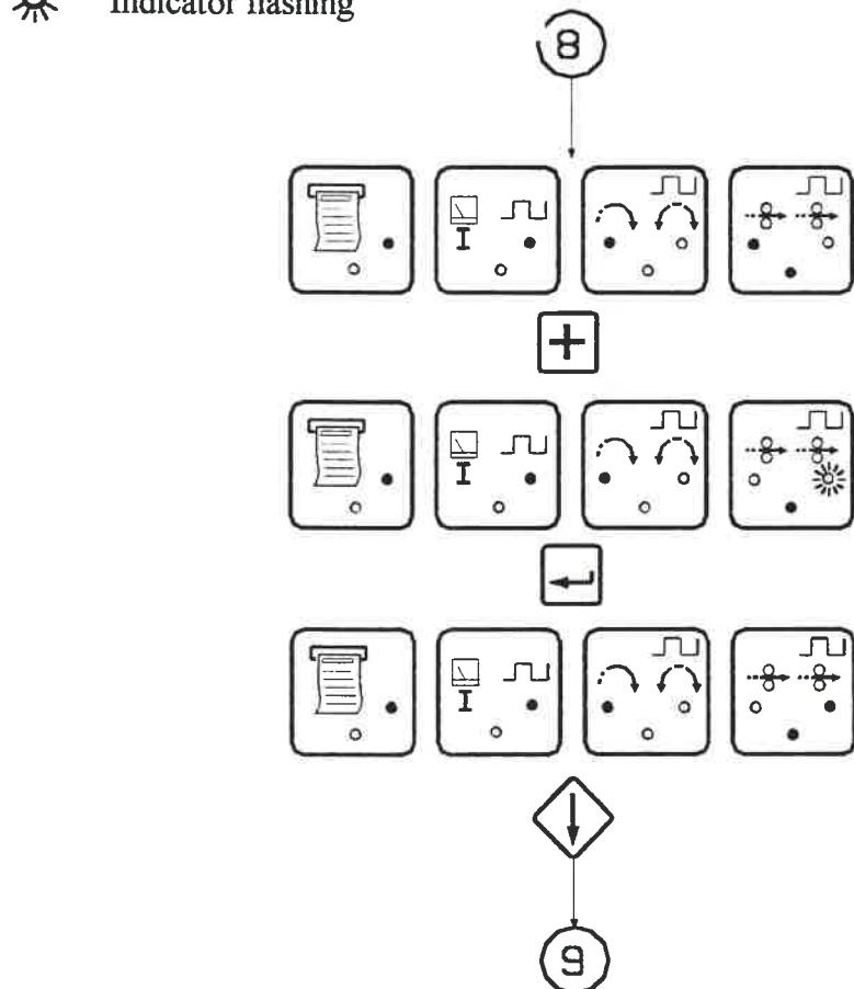
PROGRAMMING AND MODIFYING THE WELDING PARAMETERS7.2 -Gas
