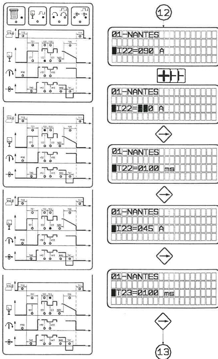
PROGRAMMING AND MODIFICATION OF THE WELDING PARAMETERS7.5 - Downslope
