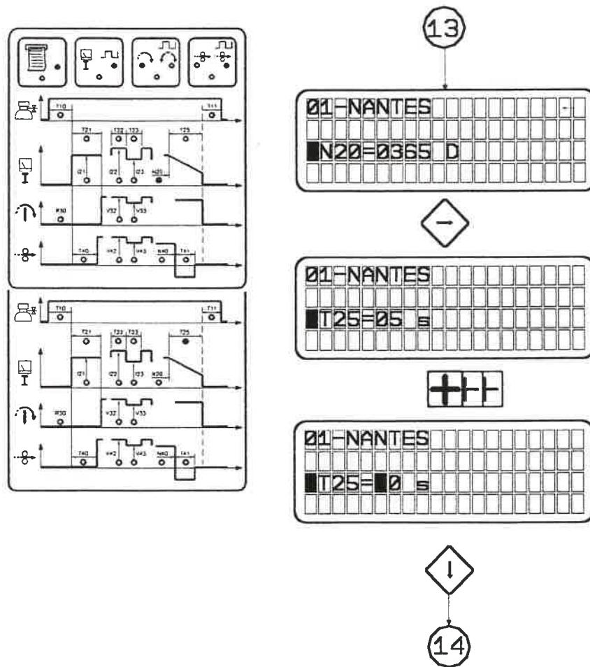
**PROGRAMMING AND MODIFICATION OF THE WELDING PARAMETERS****7.6 - Rotation; weld head reference numbers and calculation of travel speed V32 and V33****Remark**
