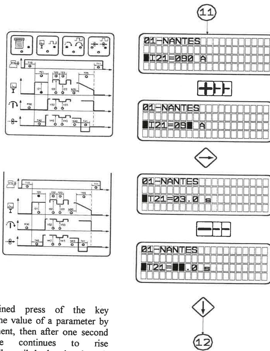
A maintained press of the key increases the value of a parameter by one increment, then after one second the value continues to rise automatically until the key is released. The value rises by one increment until the value 9 is reached, at which point it begins to rise in units of ten.
