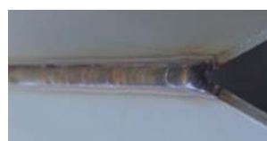
High frequency pulse for perfect corner welds
