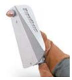
Gouging heat shield Additional protection when gouging.
