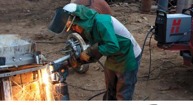
The premier system for cutting 25 mm, the Powermax85<sup>®</sup> has the same features and options as the Powermax65, but with more power from a max output current of 85 amps. A variety of Duramax<sup>®</sup> torch styles provide exceptional versatility for hand cutting or gouging, portable automation, X-Y table and robotic cutting or gouging.
