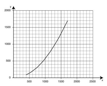
X: airflow, m³/h, Y: static pressure Pa
