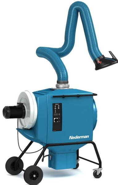
The FilterBox 12A is equipped with a powerful fan for a maximum air flow capacity of 1 200 m<sup>3</sup>/h (700 CFM). An integrated silencer reduces noise from the fan and outlet air. The unit has an advanced filter control system with automatic cleaning that starts when the air flow is too low. Available either as a mobile unit on wheels or attached to a floor stand. Additional protection from harmful particles is provided if a HEPA filter is installed.
