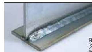
Smooth current MAG welding with flux-cored wire.
