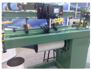
These seamers are designed for straight line welding of all weldable metals of thickness from 0.1mm to 10mm. It provides 100% penetration, single pass weld on un-tacked cylinders and flat sheets without heat distortion to the material. This optimises any process which reduces welding costs and improves the quality of the weld.
