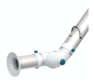
Nederman FX2 arms are made of lightweight anodized aluminium sections, with three adjustable, composite friction joints. Offering strength and durability combined with easy handling, they can be used in many types of environment. They are especially suitable for applications where small, flexible and easy-to-use arms are required.
