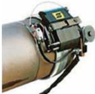
A21 PRD 100 Welding head is designed for high precision, and quality. It is a TIG welding head for tubes with an outer diameter of 100 mm or higher. Due to compact design and low profile it requires only 73 mm clearance around the tube. This is water-cooled welding head usable up to 400A.
